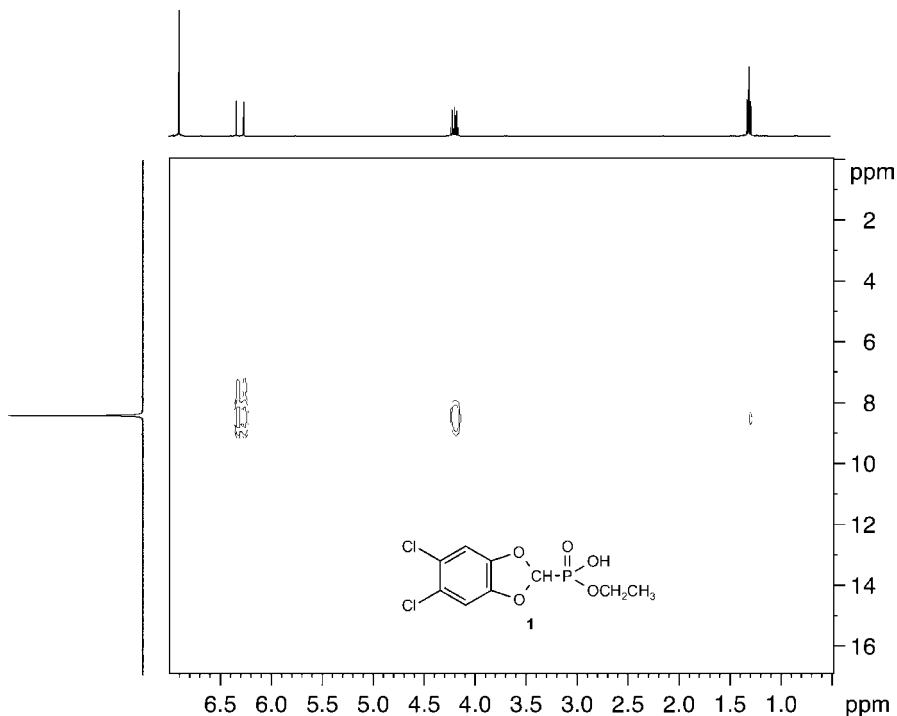
Fig. 26 P,H correlation spectrum of compound 1 (400 MHz, 5% in \text{CDCl}_3 , delay set for J_{\text{PH}} = 1.65 Hz, measurement time 12 min)
